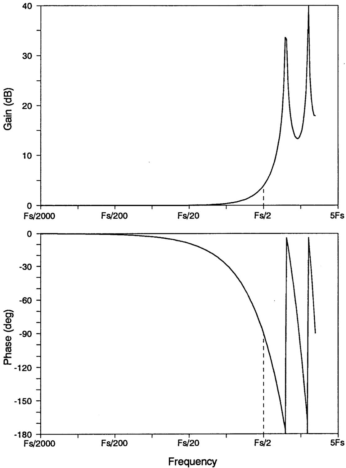
**Figure 4.1.** *Exact Transfer Function for Sampling Gain:* At half the switching frequency the gain has increased by about 4 dB, and the phase shows exactly 90° lag. High-Q poles are apparent at the switching frequency and twice the switching frequency.
