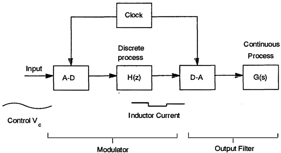
**Figure 3.7. Standard Configuration of a Computer-Controlled System:** The small-signal representation of the sample-and-hold system is shown, and the analogy with current-mode control is illustrated. The analytical results for computer-controlled systems are directly applicable to current-mode control.
