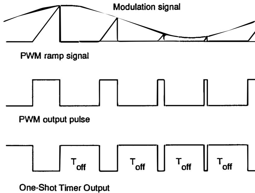
**Figure 3.9. Constant Off-Time Modulator Waveforms:**
