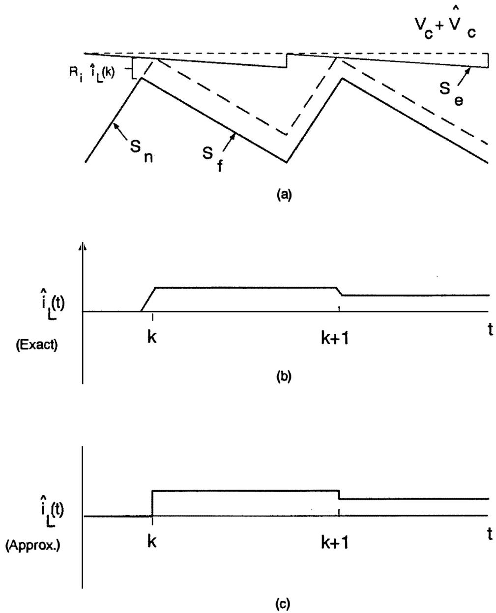
**Figure 3.6. Constant Frequency Controller with Control Perturbation:**
