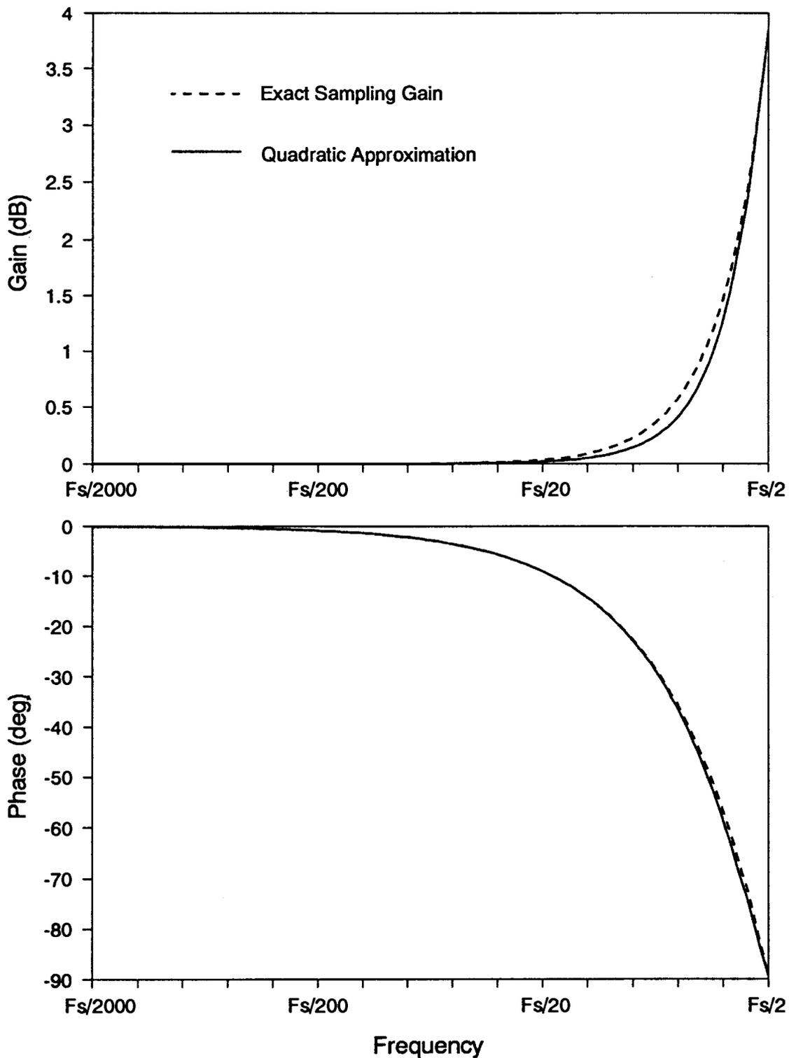
**Figure 4.3. Exact Sampling Gain and Approximation:** *The approximate sampling gain expression, given by a quadratic formula, is equal to the exact expression at dc and half the switching frequency, and differs by less than 0.2 dB and 3 degrees at all frequencies in between.*
