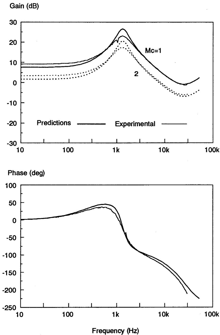
**Figure 5.5. Buck Converter Current Loop Gain - Experimental Results:** The predicted and experimental results for the current loop gain agree very well, especially at higher frequencies where average models fail to predict the current-loop instability.
