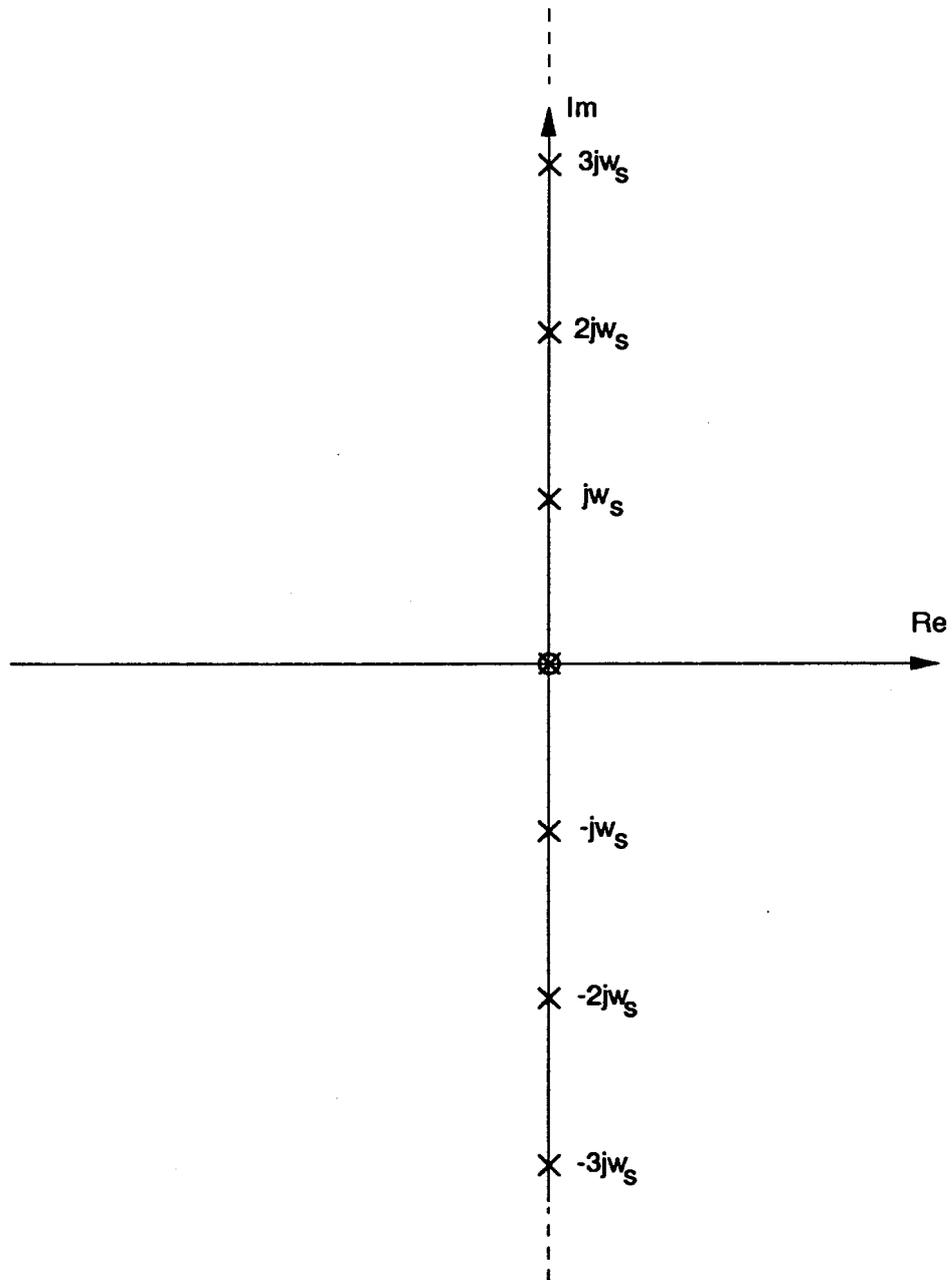
**Figure 4.2.** *Pole-Zero Locations of the Exact Sampling Gain: The exact sampling gain transfer function has a pole and a zero at the origin, and an infinite number of complex pole pairs occurring at each integer multiple of the switching frequency.*
