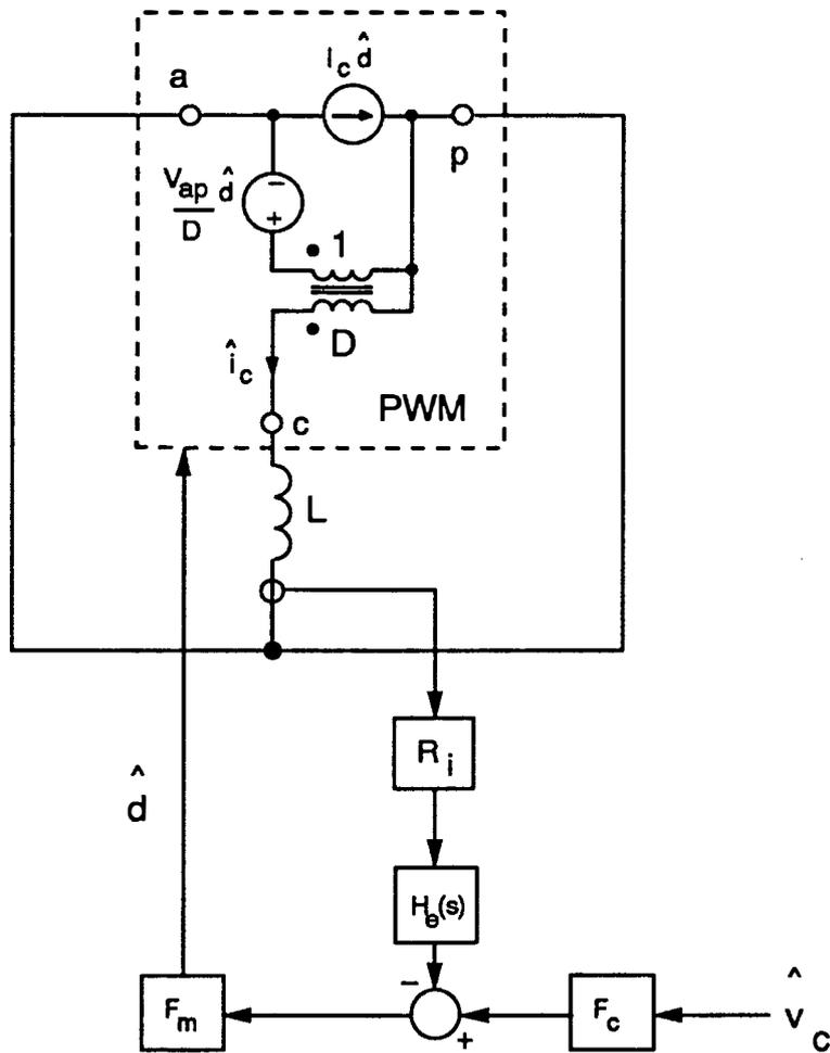
**Figure 3.4. Small-Signal Model of the Current-Mode Cell with Fixed Voltages:**
