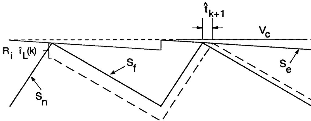
**Figure 3.8. Current-Mode Control Modulator with Perturbation in Current:**
