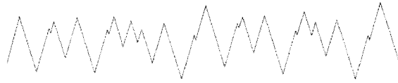
Figure 9: Inductor current waveforms at D=0.44 , with outer feedback loop closed. System is now unstable, as shown by the loop gain of Fig. 7. A plot without the double pole extension to the model does not predict this oscillation.
